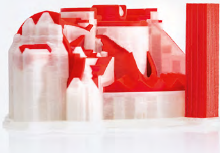
Model of gear mechanism before support material dissolution
