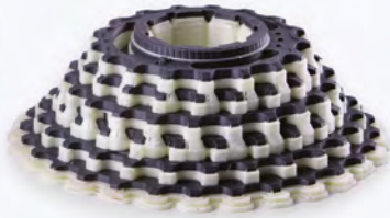
Bicycle cassette model before support material dissolution
